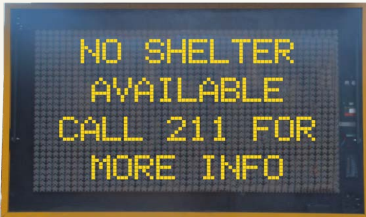
LA DOTD uses Variable Messaging Signs (VMSs) to send messages to drivers.
